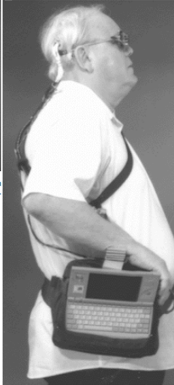
Figure 1. Blind volunteer with sub-miniature TV camera mounted on the right lens of his sunglasses, and the laser-pointer (position monitor) on the left temple piece.
