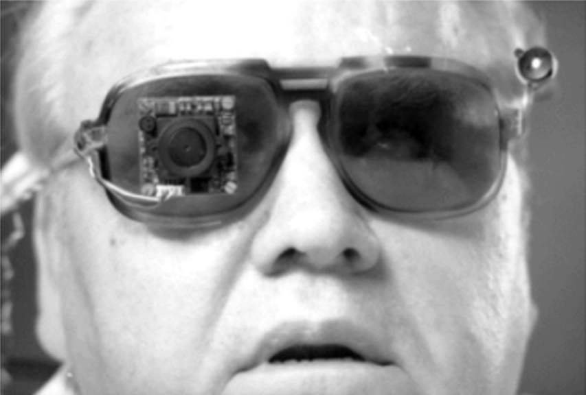
Figure 1. Blind volunteer with sub-miniature TV camera mounted on the right lens of his sunglasses, and the laser-pointer (position monitor) on the left temple piece.
